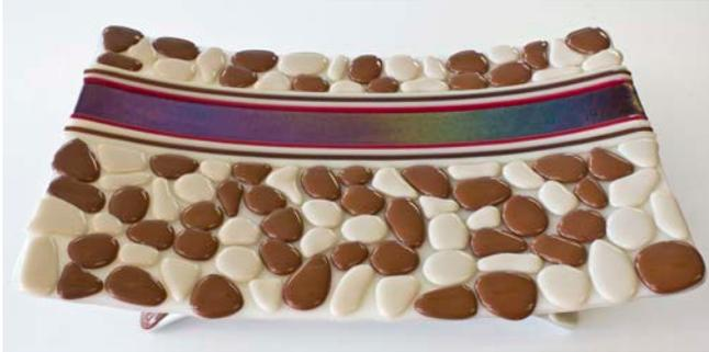
*Both the fuse and the slump and drape firings of this tray made with pre-made full fused ¼" thick nuggets and strips of glass rod on a ¼" base were ramped at 75°F to allow even heat transfer through the glass. This was ½ inch thick at thickest point and ¼" at thinnest. If it had been a uniform ½ inch it could safely have ramped at 200°F. Uneven thickness required a much slower ramp speed.*
