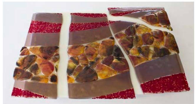
*The tack fuse firing of this project with pre-fused 1/4" thick nuggets made from pieces of a broken up screen melt on a 1/4" thick base was at 150°F per hour. Even at that low ramp speed, the kiln heat failed to transfer evenly through the glass and it cracked on the ramp up*
